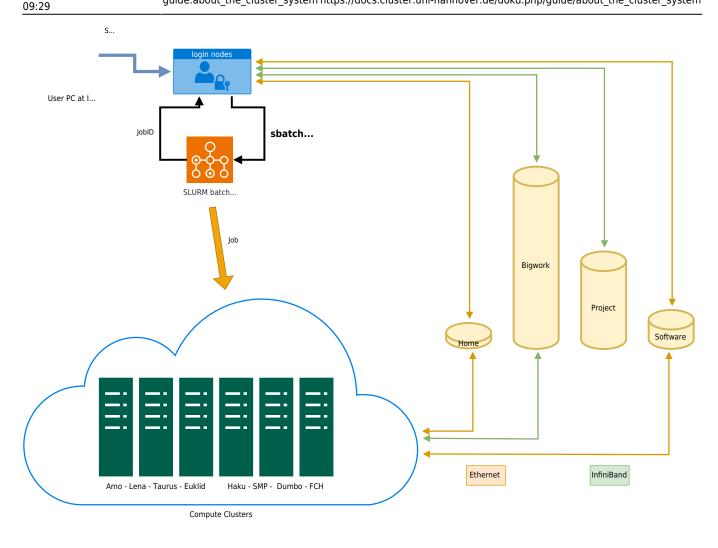
Fig. 1: Sketch of the main user-relevant components of the cluster system
